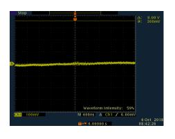
Fig.1 Measurement of ambient noise of an ethernet port with power off.
