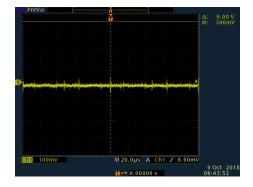
Fig.3 Measurement of an ethernet port with the VFD powered on; while using an Enerdoor EMI filter.
